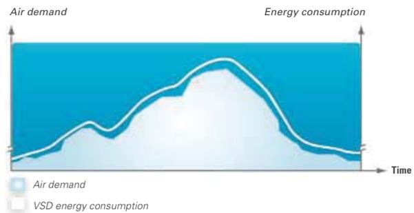
Traditional compressors working with a full load, no load control operate between two set pressure points. When maximum pressure is reached the compressor goes off load. During periods of medium to low air demand, the no load power consumption can be excessive – wasting large amounts of energy.
